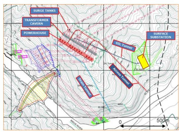
Fig 3.2: Alignment of Power House Complex
