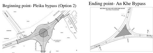
Figure 2 -Design of Intersections with Measures to Ensure Traffic Safety
