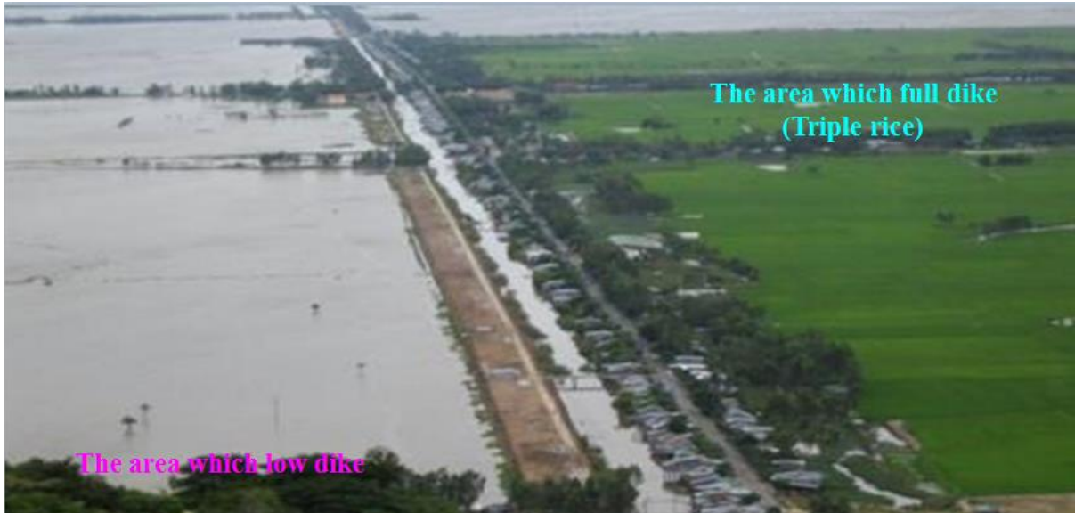
Figure 40: The inundation status at main flood season (the right area which full dike and the left which low dike)
