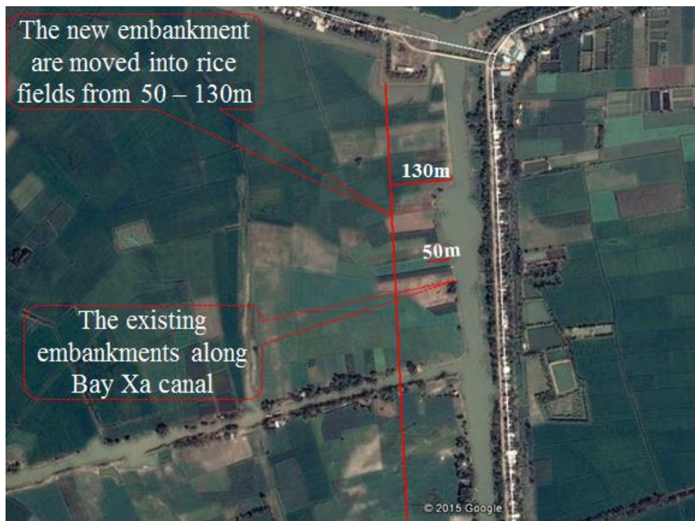
Figure 51: Plan of dikes along the 7 communes canal compared to the existing dikes
