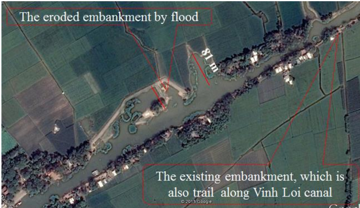
Figure 44: Erosion on Vinh Loi canal
