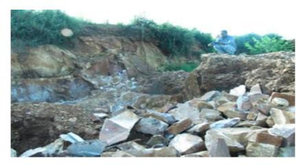
Plate 3-4: Munege rock quarry, Km 20+100, RHS, Offset 300m (Whitish grey quartzite and granitic)
