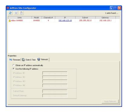
You must change your own IP address so that you can reach the IP address 192.168.123.10. When you run the ioiWare Site-Configurator, it detects the device. Select the device and then the Network tab. You can configure the device's IP address to be static or obtain an IP address automatically. When finished, click Apply Network.
