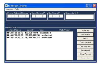
Click Find Cameras to search for Arecont IP cameras on the local subnet. If the program does not detect the camera, verify that the cameras are actually in your local subnet.
