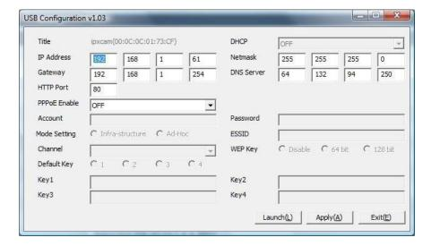
Select OFF from the DHCP drop-down list in the utility. Enter the IP address, netmask, gateway, DNS server, and HTTP port information. Click Apply and then Exit when finished.
