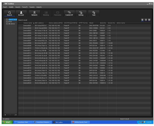
Select the camera to edit the camera IP properties. Sony cameras typically do not use DHCP by factory default, you must manually assign the camera an IP address. Enter an IP address that is not used by any other device on your local network, ensuring that the first three numbers match the first three numbers of your exacqVision Server's IP address. Set the subnet to 255.255.255.0, leave the HTTP port at 80, enter the camera's Administrator name and password, and click Apply.
