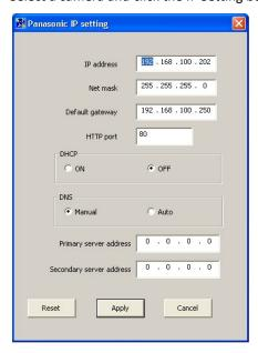
Panasonic cameras typically do not use DHCP by factory default, you must manually assign the camera an IP address. Enter an IP address that is not used by any other device on your local network, ensuring that the first three numbers match the first three numbers of your exacqVision Server's IP address. Set the net mask to 255.255.255.0, leave the HTTP port at 80, enter the camera's Administrator name and password, and click Apply.
