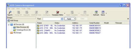
AXIS cameras on the network are listed. Right-click a camera and select Enter Device Credentials....
