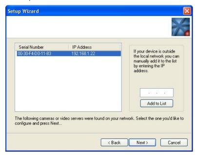
Select the method used to connect to the camera and then click Next. Select the IP camera from the list and click Next. The configuration of the camera is then displayed. Select the primary method of communication, which is usually Network.
