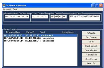
Click Set IP to set the IP address. To configure additional information for the camera, go to the camera's web page.
