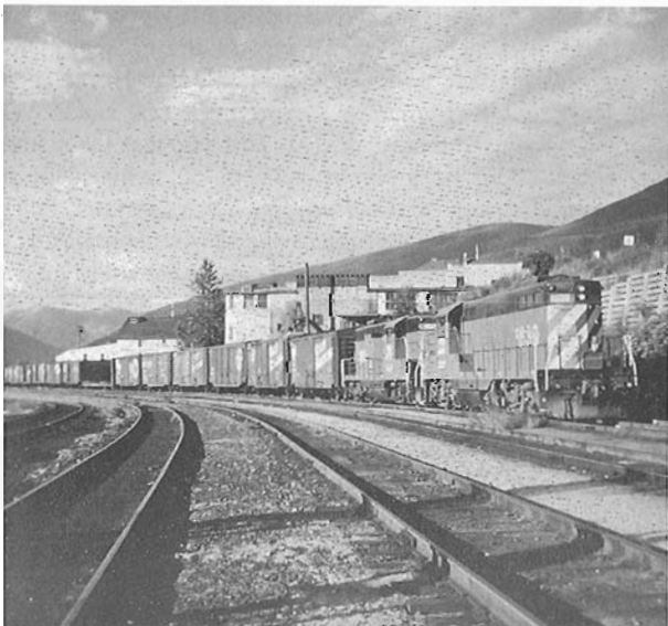
BN 1839 and 1832 enter the Nelson yard about 7:30 pm on a warm July evening in 1971. The engines will back the rather typical consist, into the siding behind the train, this was standard procedure and then be parked on the shop track to the left of the picture for servicing. 1839 is X GN 687. 1832 well also be an X GN engine but I have not been able to track down its number. Photo by author.
