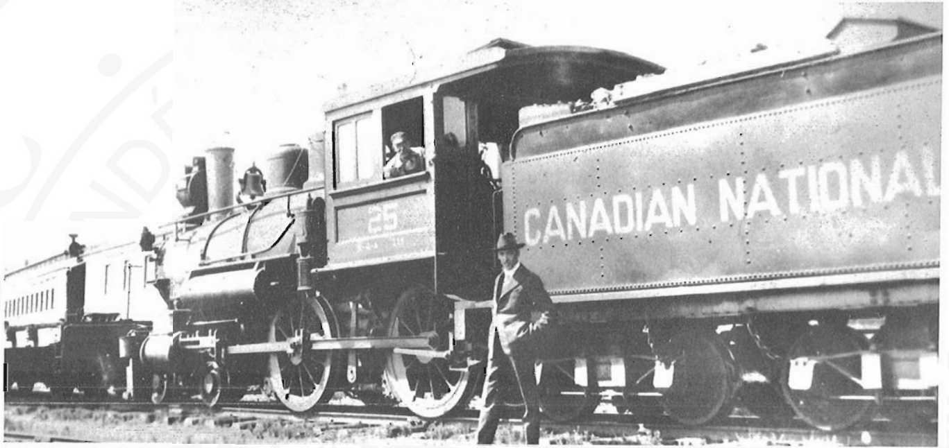
Canadian National had narrow gauge locomotives on its roster many years before it took over the Newfoundland Railway. CN 25, a 4-4-0, was built by the Canadian Locomotive Works at Kingston, Ontario for the Prince Edward Island Railway in 1901. Rendered obsolete by the introduction of standard gauge operations, it was one of 9 narrow gauge 4-4-0's retired by CN in 1923.
