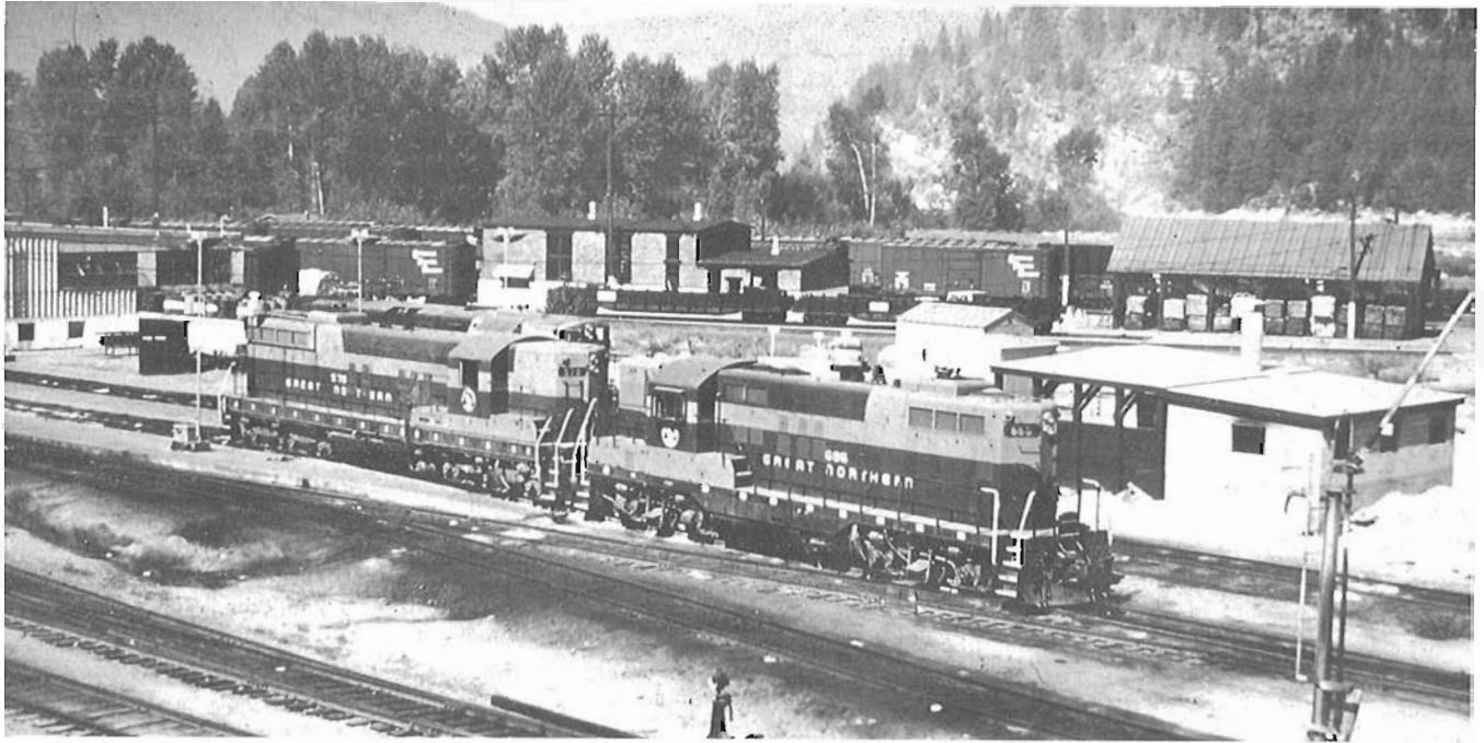
GN SD9 #578 and GP9 #686 sit on one of the shop tracks in Nelson. It was generally difficult to get photos of these engines in Nelson because the train arrived in the evening and left early in the morning. For some unknown reason the train arrived mid morning and left mid afternoon on this occasion. These engines were regulars on the run for many years. Often the SD9 was the only power necessary. The 686 became BN 1838 that remained in service on the line until recently. John Rushton Photo. Mid 1960's.
