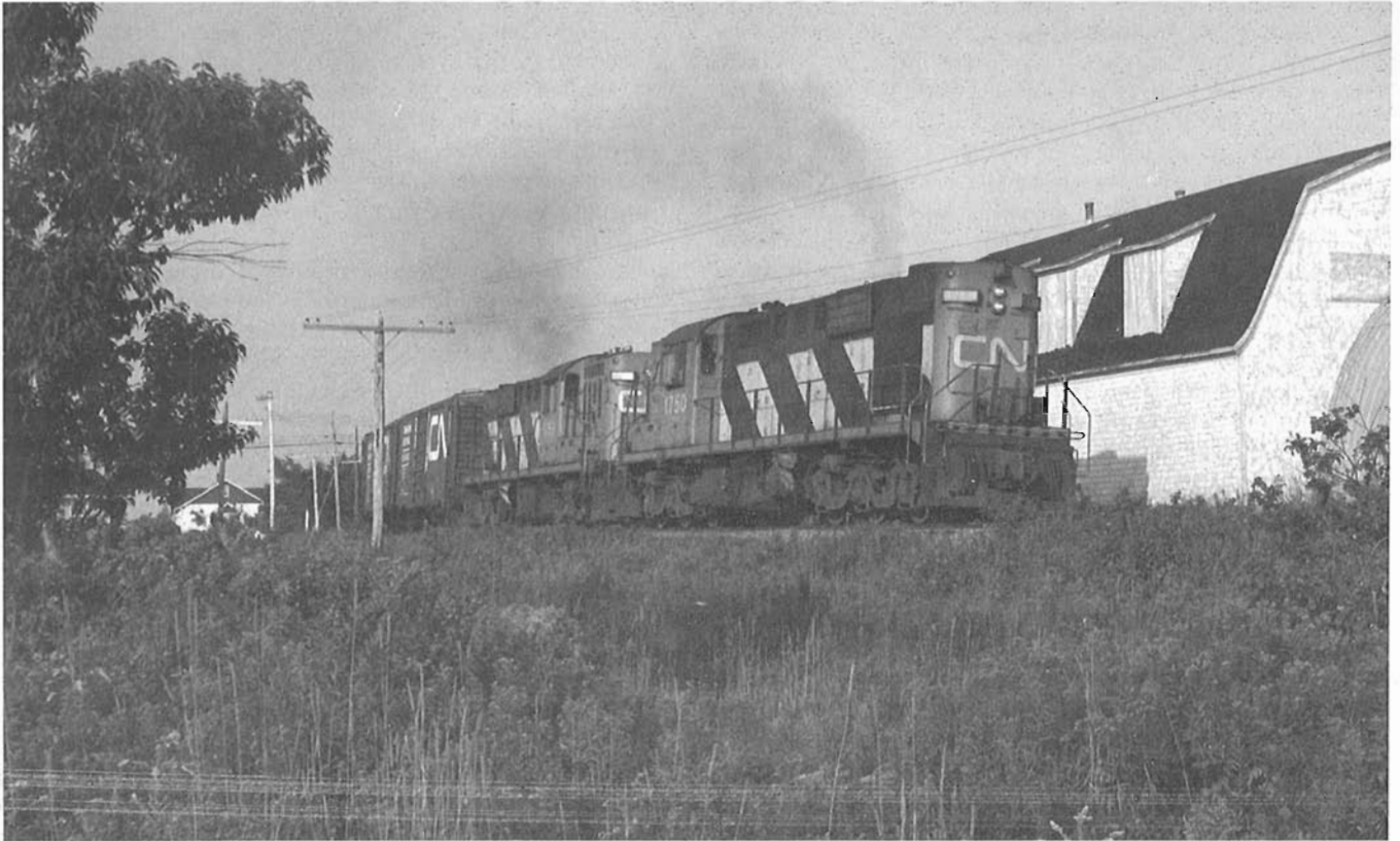
In 1975 and 1976, CN converted a number of its RS-18m units into RSC-14's for service on lightweight rail lines. The original B-B wheel sets were replaced with A-1-A wheel sets and the horsepower was reduced from 1800 to 1400. In September 1982, two of these rebuilt units, the 1750 and 1753, were highballing a freight from Borden to Charlottetown. A quick moving train and a lack of intermediate switching meant only one photograph was possible between Emerald Junction and Charlottetown. The building along the track is one of the potato warehouses which at one time provided the major source of traffic for the railway.
