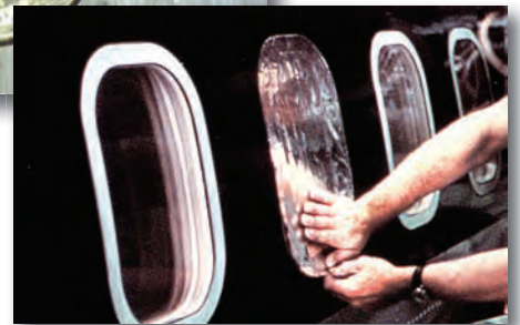
With conformability and chemical resistance, die-cut masks of 3M™ Aluminum Foil Tape protect aircraft windows during harsh chemical paint stripping.
