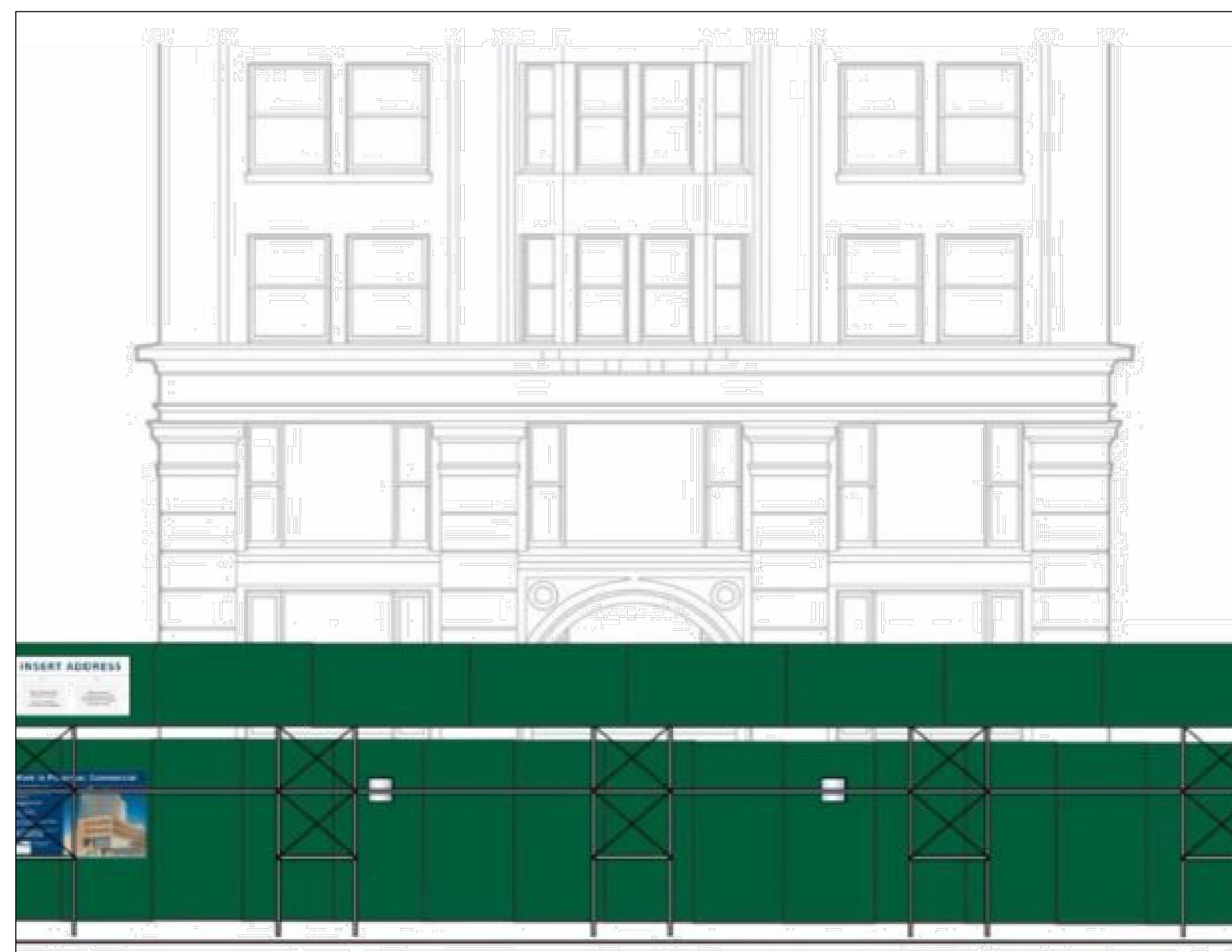
PROJECT INFORMATION PANEL AND SIDE WALK SHED PARAPET POSTING
