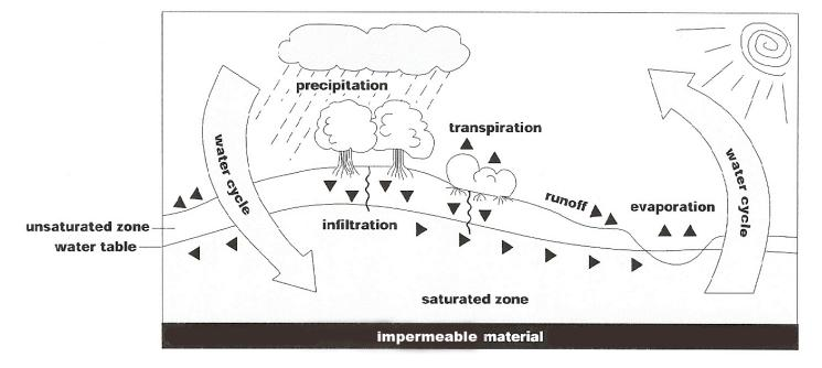
Figure 1. In the water cycle, precipitation that falls may run off into the stream (runoff) or soak into the ground (infiltration). Some of the water that falls, returns to the air by evaporation or passing through plants (transpiration). Water pulled through the soil by gravity into the saturated zone becomes groundwater.
