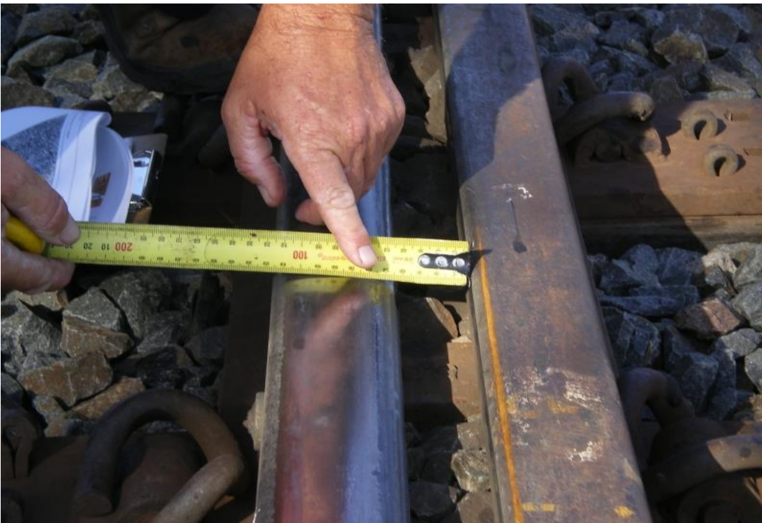
Photo 6 Measuring Flangeway Clearance
