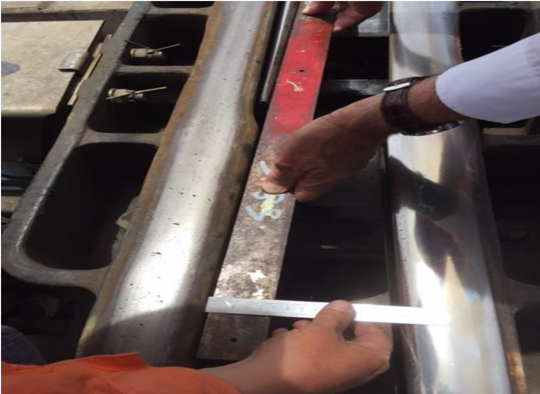
Photo 10 Straight edge on running face with SNX in the normal position
