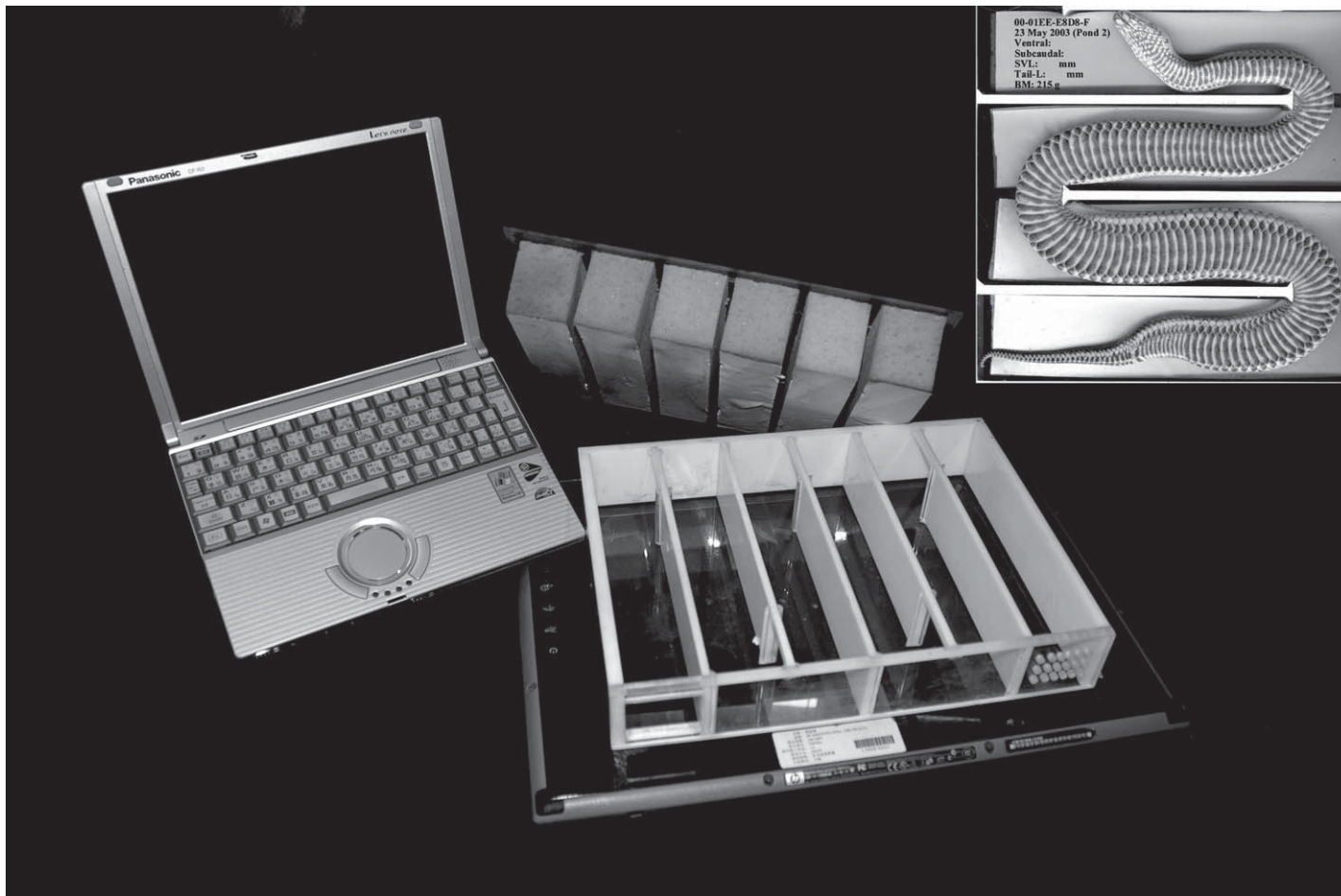
FIG. 1. The scanner platform module (the main figure) from left to right clockwise; the PC notebook, cover glued with six sponge strips, the white labyrinth with one transparent side for animal observations, and a HP-4670 scanner. The upper right insert is the ventral image of an Enhydryis chinensis with a tag number, indicating the collection and measurement data.
