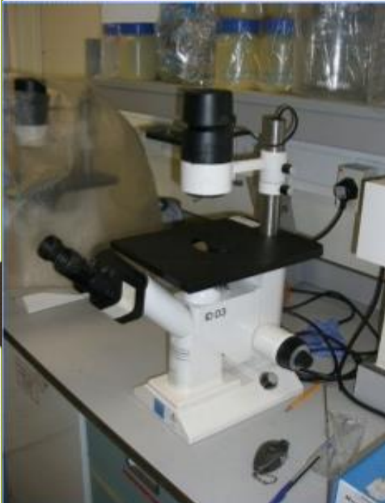
Microscope Large stage so plates and flasks can be used. Magnification; 5X, 10X, 20X, 40X
