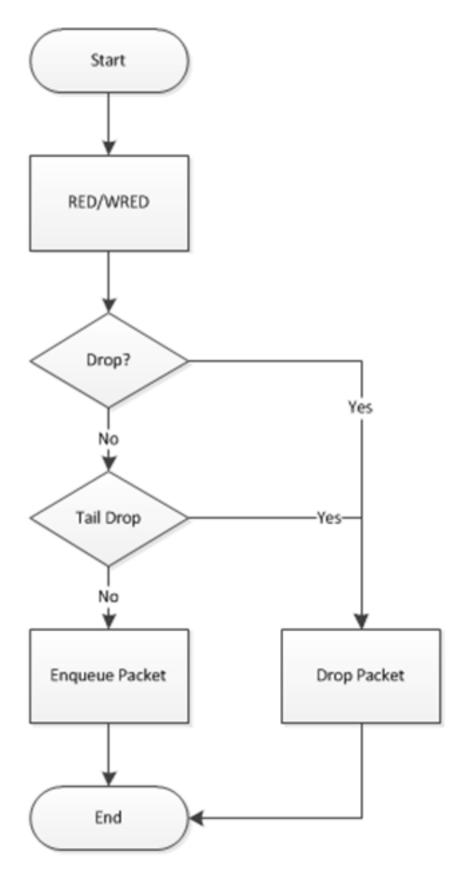
Fig. 23.8: Flow Through the Dropper
