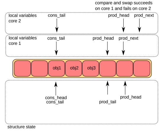
Fig. 4.9: Multiple producer enqueue second step
