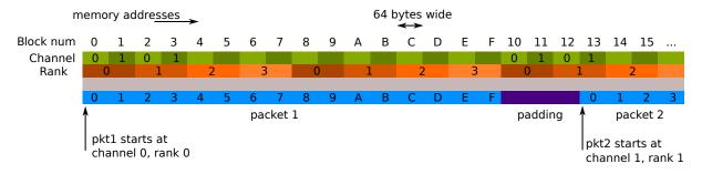
Fig. 5.1: Two Channels and Quad-ranked DIMM Example
