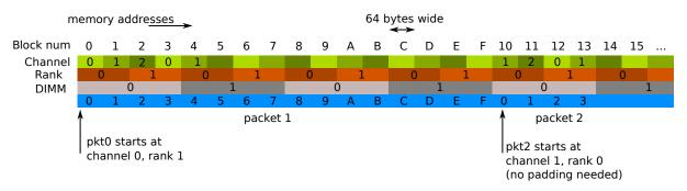
Fig. 5.2: Three Channels and Two Dual-ranked DIMM Example
