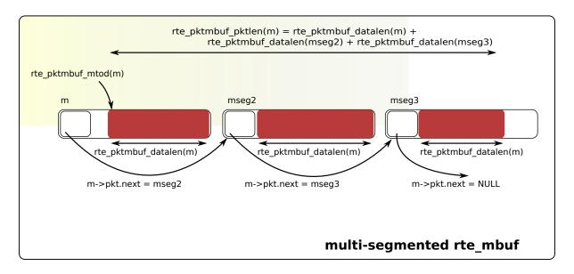
Fig. 6.2: An mbuf with Three Segments
