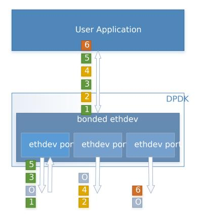
Fig. 10.6: Link Aggregation 802.3AD (Mode 4)
