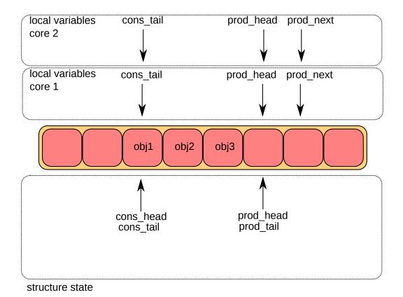
Fig. 4.8: Multiple producer enqueue first step
