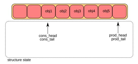
Fig. 4.12: Multiple producer enqueue last step
