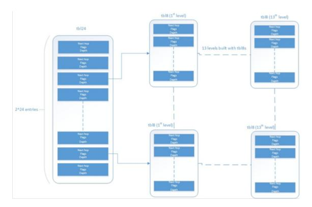
Fig. 15.1: Table split into different levels
