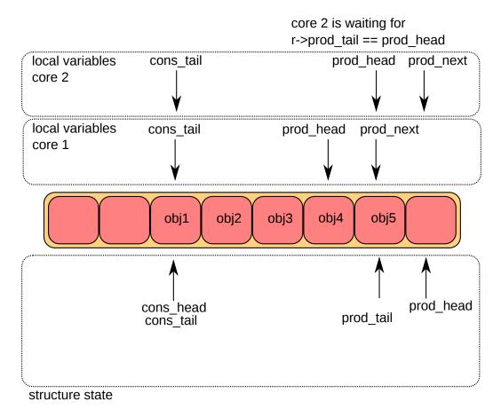
Fig. 4.11: Multiple producer enqueue fourth step
