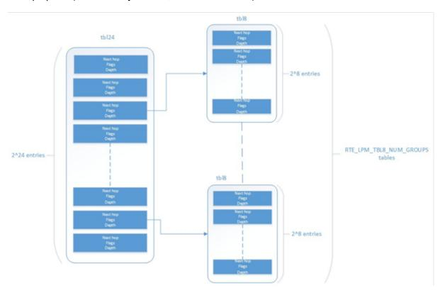
Fig. 14.1: Table split into different levels
