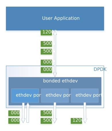
Fig. 10.7: Transmit Load Balancing (Mode 5)
