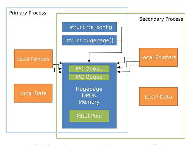
Fig. 20.1: Memory Sharing in the DPDK Multi-process Sample Application
