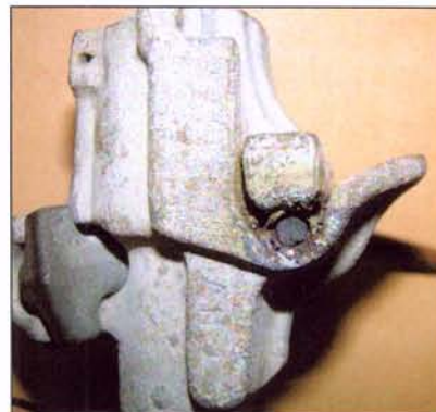
Figure 2: View of fractured conductor in hot tap saddle
