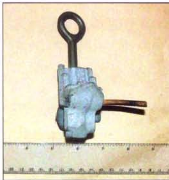
Figure 1: Hot tap and failed #4 AWG conductor received for examination
