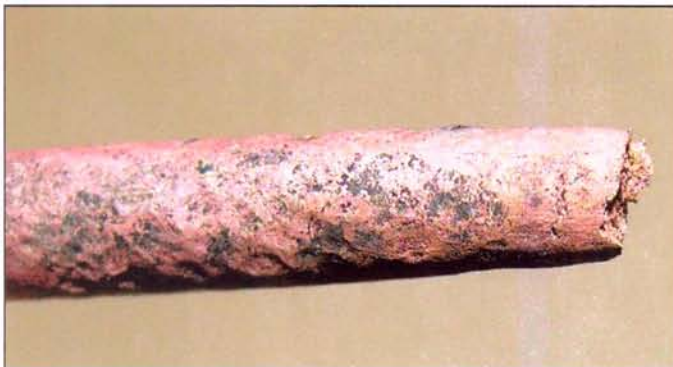
Figure 7: Macro image of surface condition of failed copper conductor
