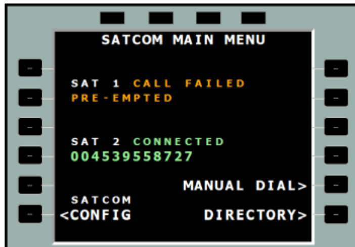
Figure 7-22: MCDU - SATCOM Main Menu - Call failed - Pre-empted
