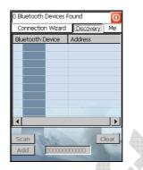
Once the Discovery procedure has been completed, select the desired Bluetooth® device from the list. It is also possible to digit (12 hexadecimal digits) the Bluetooth® address of the desired device by tapping on the "Add" button. The "Clear" button deletes all discovered devices from the list.
