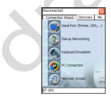
The "Serial Port" button starts communication through the Bluetooth $\circledast$  serial port COM 5 (typically used for connection with GPS devices).
