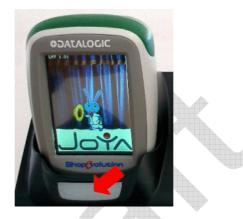
If user does not insert Joya into a slot, a timeout message is displayed asking to remake the operation. In case of errors a suitable message is displayed.
