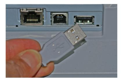
The power supply for the MiCard® reader is provided via the USB connection.
