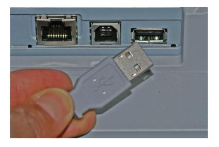
The power supply for the MiCard® reader is effected via the USB connection.
