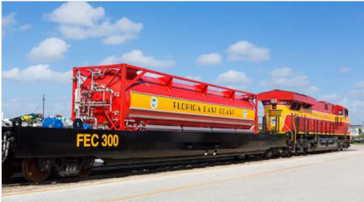
Figure 2-34 | Florida East Coast Railway LNG Fuel Tender and Locomotive
