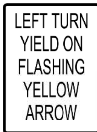
Figure 3.10-3. Flashing Yellow Arrow Sign (FTP-85-13)
