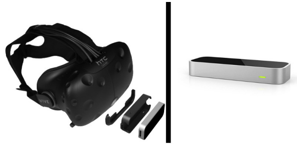
Figure 2.16: Headset Vive with mounted Leap Motion sensor on the left and Leap Motion Controller on the left
