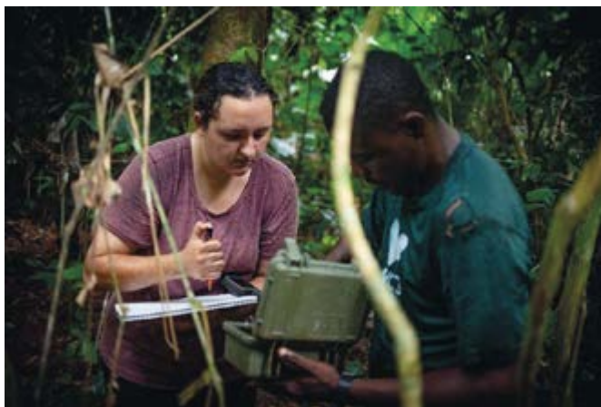
Anahita setting up an acoustic recording unit during fieldwork completed in the Republic of Congo in 2021. The goal was to create an acoustic gunshot classifier that could appropriately label the sound of a gunshot that originated from an automatic vs. non-automatic gun.
