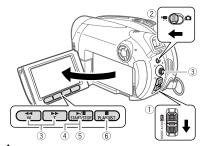
1 Move the power switch to ON, then slide it down toward MODE and release it to set the camcorder in PLAY mode.
