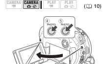
Move the power switch to ON to set the camcorder in CAMERA mode. The red CAMERA indicator will turn on.
