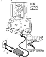
3 Connect the power cord to the compact power adapter.
