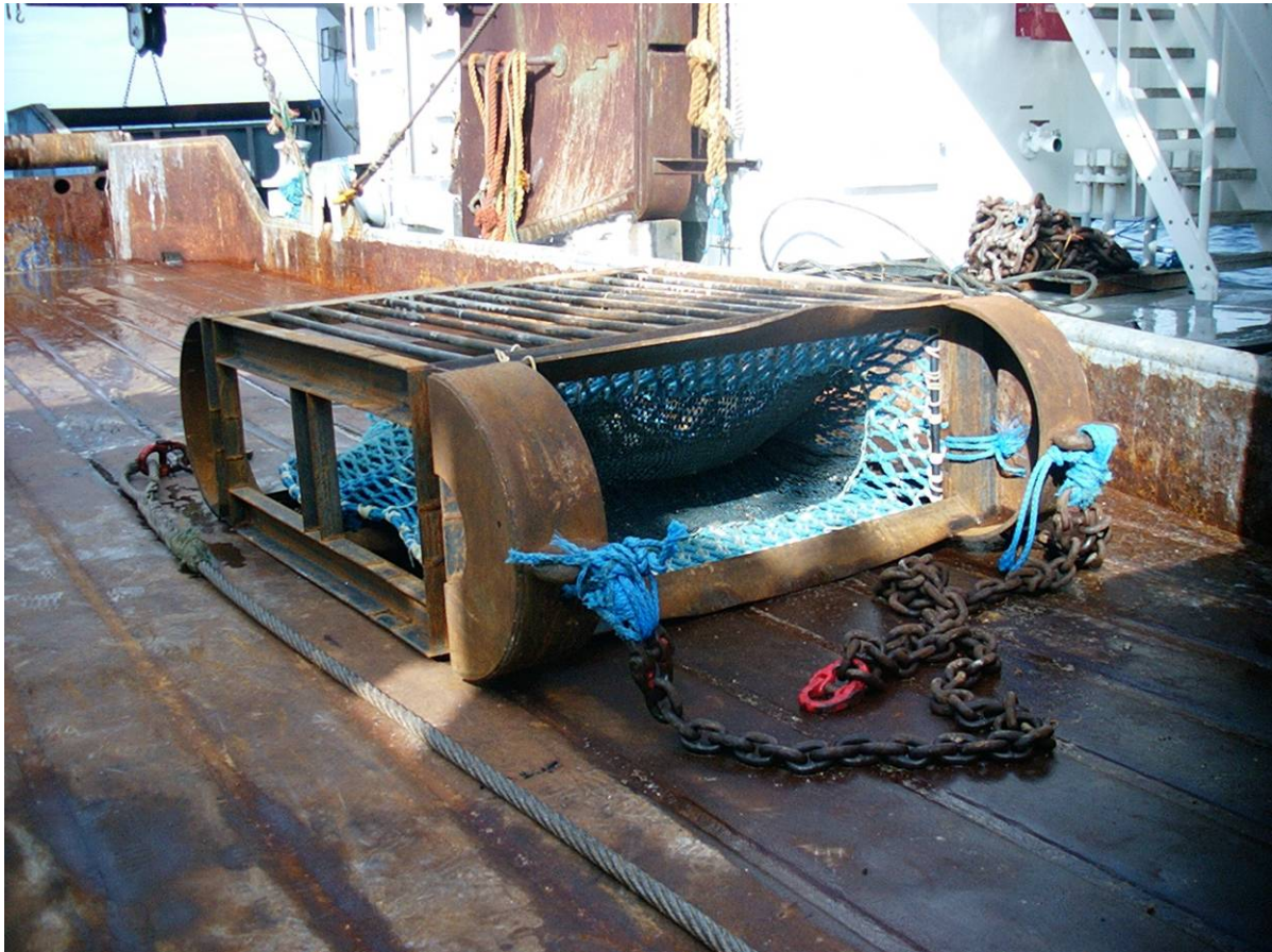
Figure 27: Seamount sled often used in New Zealand for sampling megafauna of hard substrata.
