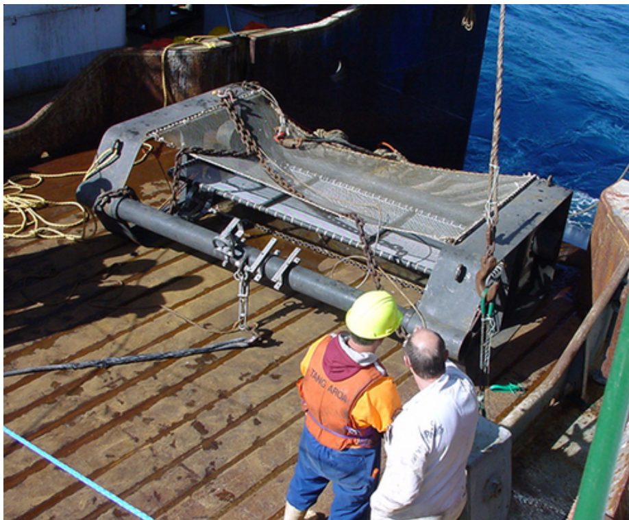
Figure 23: Agassiz trawl on deck of RV Tangaroa .
