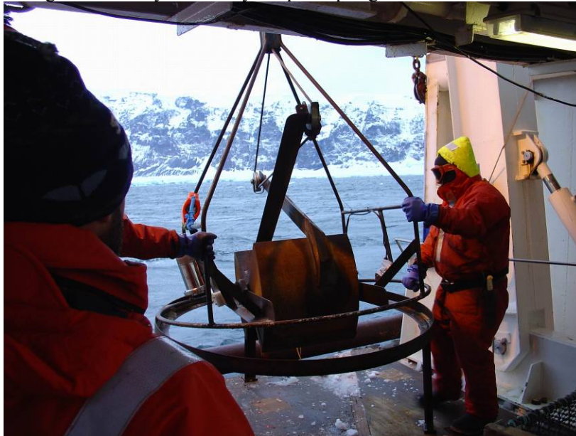
Figure 28: Large grab deployed from R/V Tangaroa in Antarctica.
