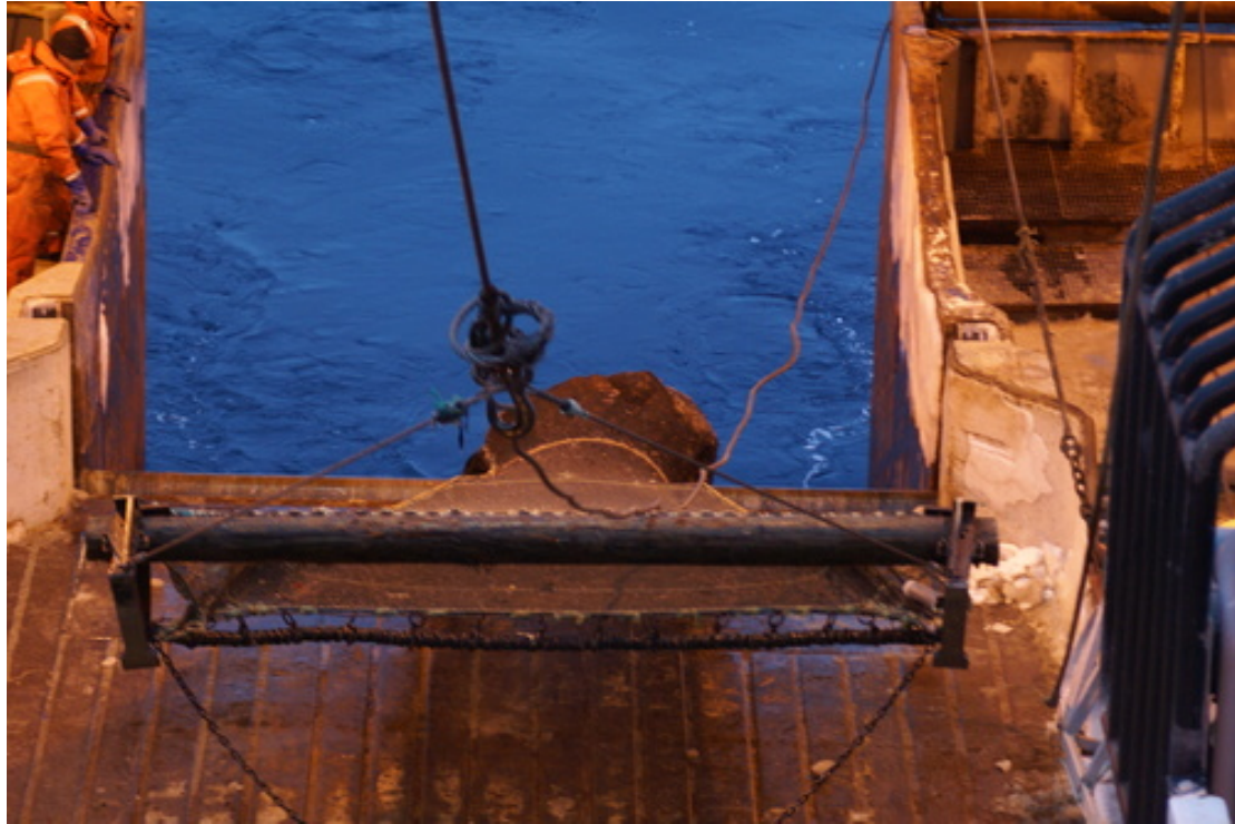
Figure 24: Beam trawl being brought on deck aboard RV Tangaroa .
