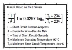
Did a comparison check - used AWG 4 cable (41783.44cmil) plugged into the above formula. Then used the equivalent 21.15mm<sup>2</sup> cable and plugged it into Eq. 1. Results differed by about 1% which I would easily ascribe to all the rounding errors I made.
