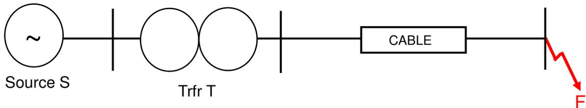
Suppose the transformer LV network is 380V. What is the minimum length of cable required to ensure that the three-phase fault current at F does not exceed the cable fault current rating for a given time?
