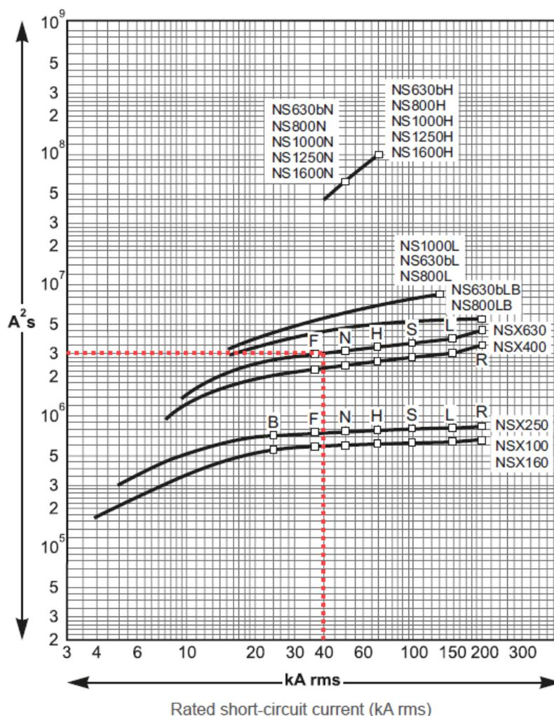
Thus, with a prospective fault current of 40kA, the maximum let-through energy of the NSX630 breaker is  $3 \times 10^6 \text{ A}^2 \cdot \text{s}$ .
