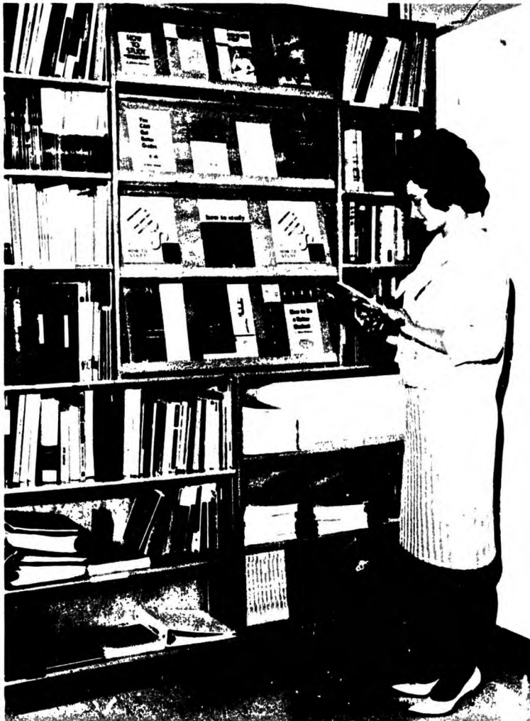
Example of guidance information unit. The sloping racks for pamphlets and magazines are of convenient height and are hinged at top to provide accessible storage space behind.
