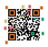
Zone 1. Position: the marks of the three corners allow the reader to locate the position of the code and start reading. It is convenient that around there is a white margin.
