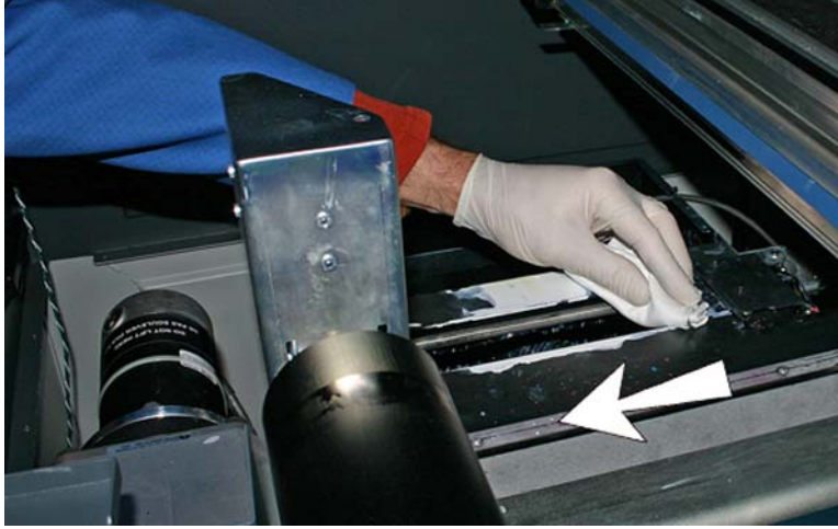
Figure 18 Cleaning the top of the service station
