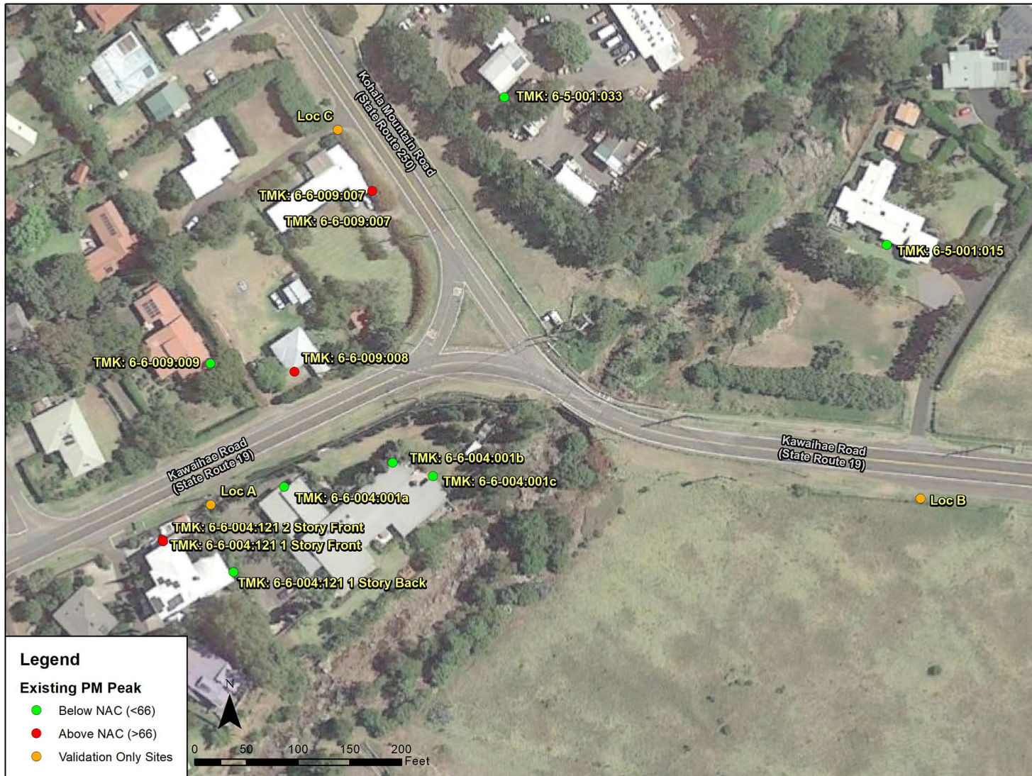
Figure 3-2. Noise Measurement and Modeling Locations and Modeled Existing Noise Levels (Kawaihae Road, Replacement of Waiaka Bridge and Realignment of Approaches)
