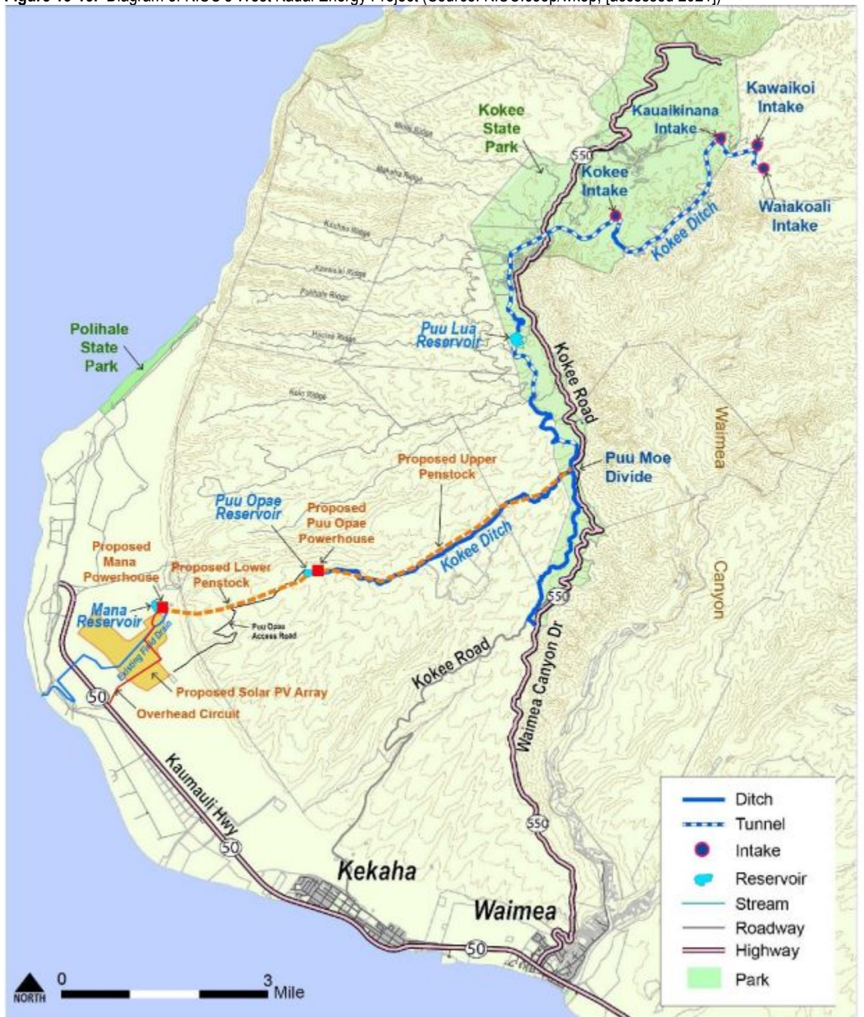
Figure 13-13. Diagram of KIUC's West Kauai Energy Project (Source: KIUC.coop/wkep, [accessed 2021])
