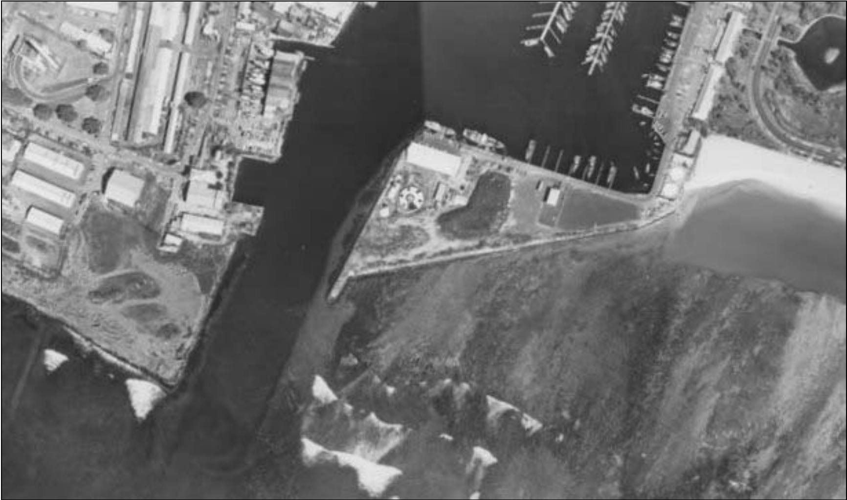
Figure 29. 1968 aerial photograph mosaic of entry to Kewalo Basin showing land fill at west side of entrance
