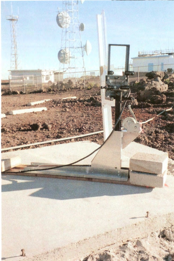
Figure 4. Vertical radar mount extended and in vertical sampling position.
