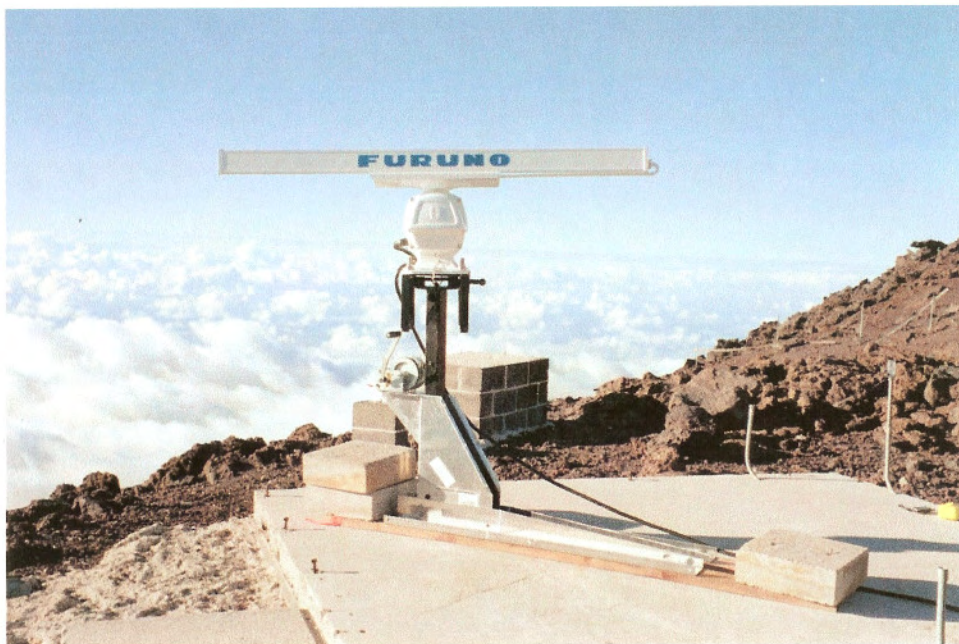
Figure 3. Vertical radar mount extended and in surveillance sampling position.
