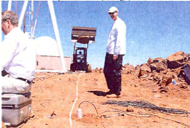
Fig. 4 - Dropping Rock for SASW Survey on Site 2 N-S with 1 Hz Geophone Pair (silver)
