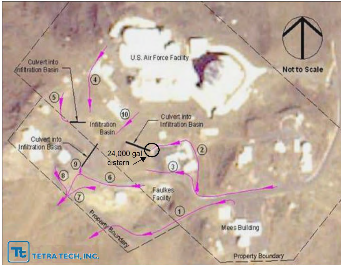
Figure 2-10. Existing Stormwater Runoff Patterns at HO.
