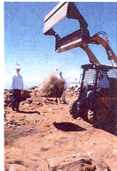
Fig. 5 - Caterpillar 226B Loader dropping ~600 lb Boulder for SASW tests
