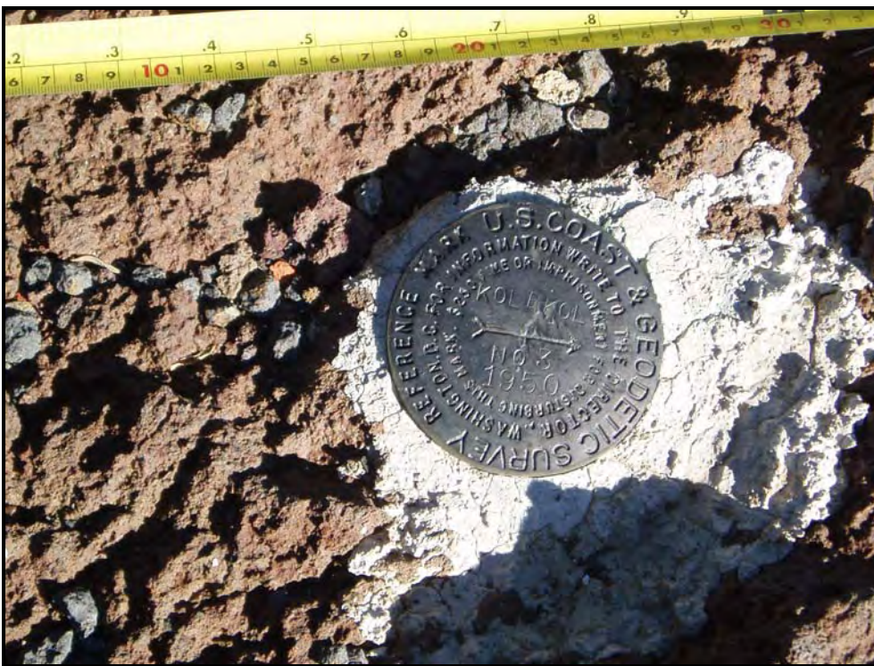
Photograph 5: View of a Reference Mark—US Coast & Geodetic Survey disc (dated 1950).
