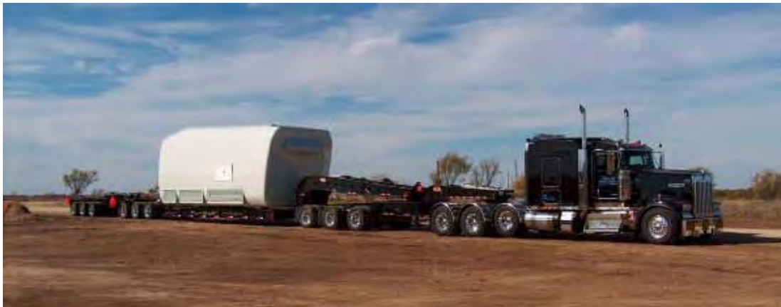
Figure 3.9-3. Typical Nacelle 13-Axle Combination Transport
