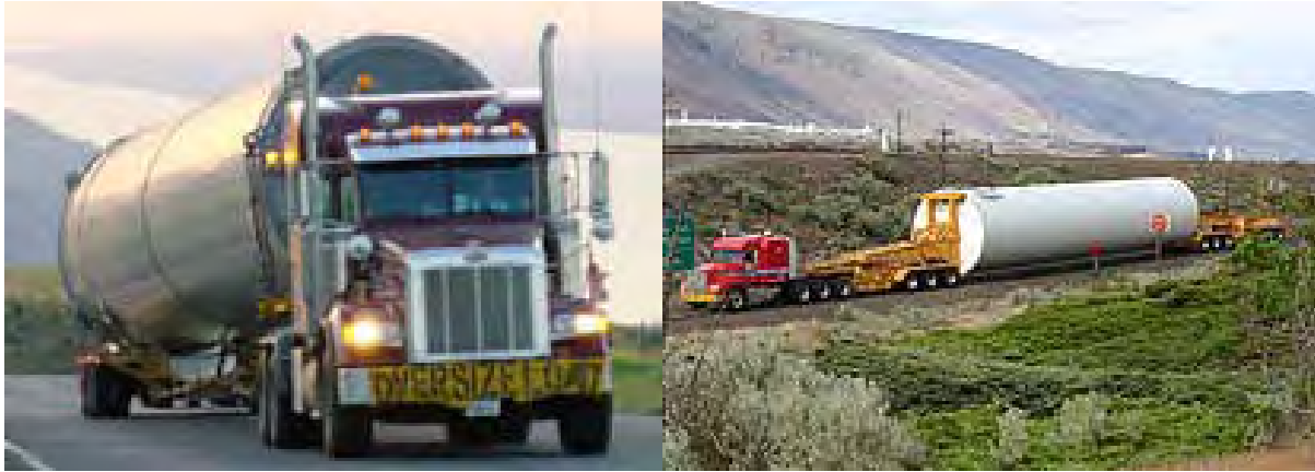
Figure 3.9-4. Typical WTG Tower Transport
