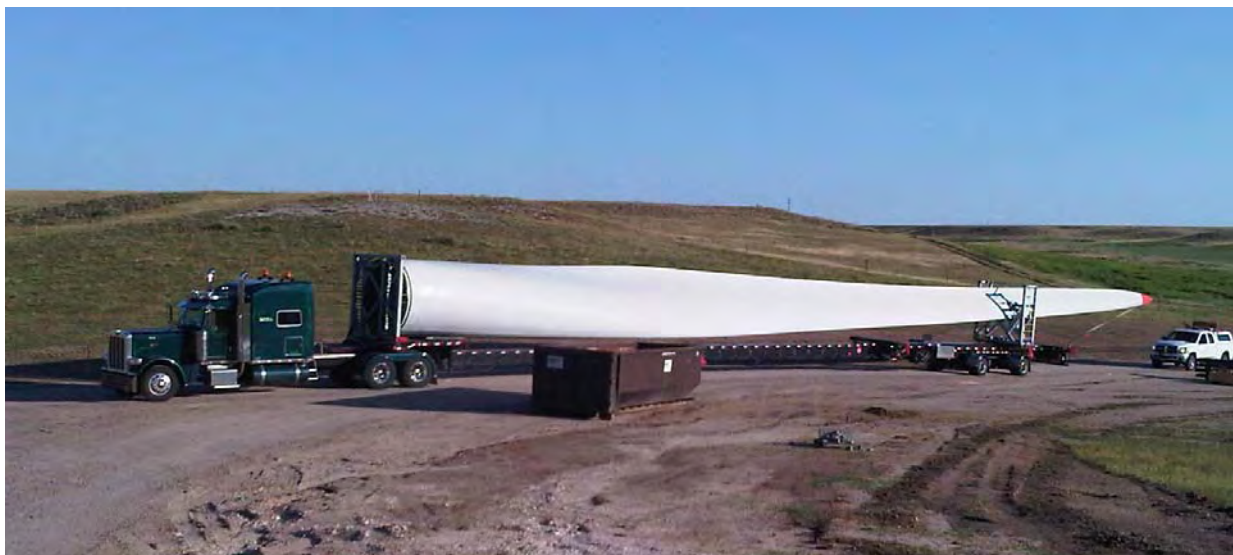
Figure 3.9-5. Typical Blade Transport
