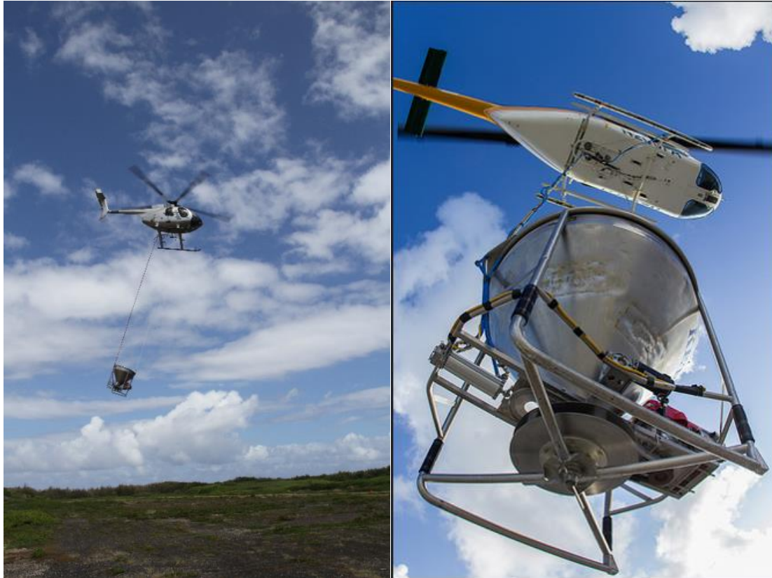
Figure 2: Hopper suspended from a helicopter.
