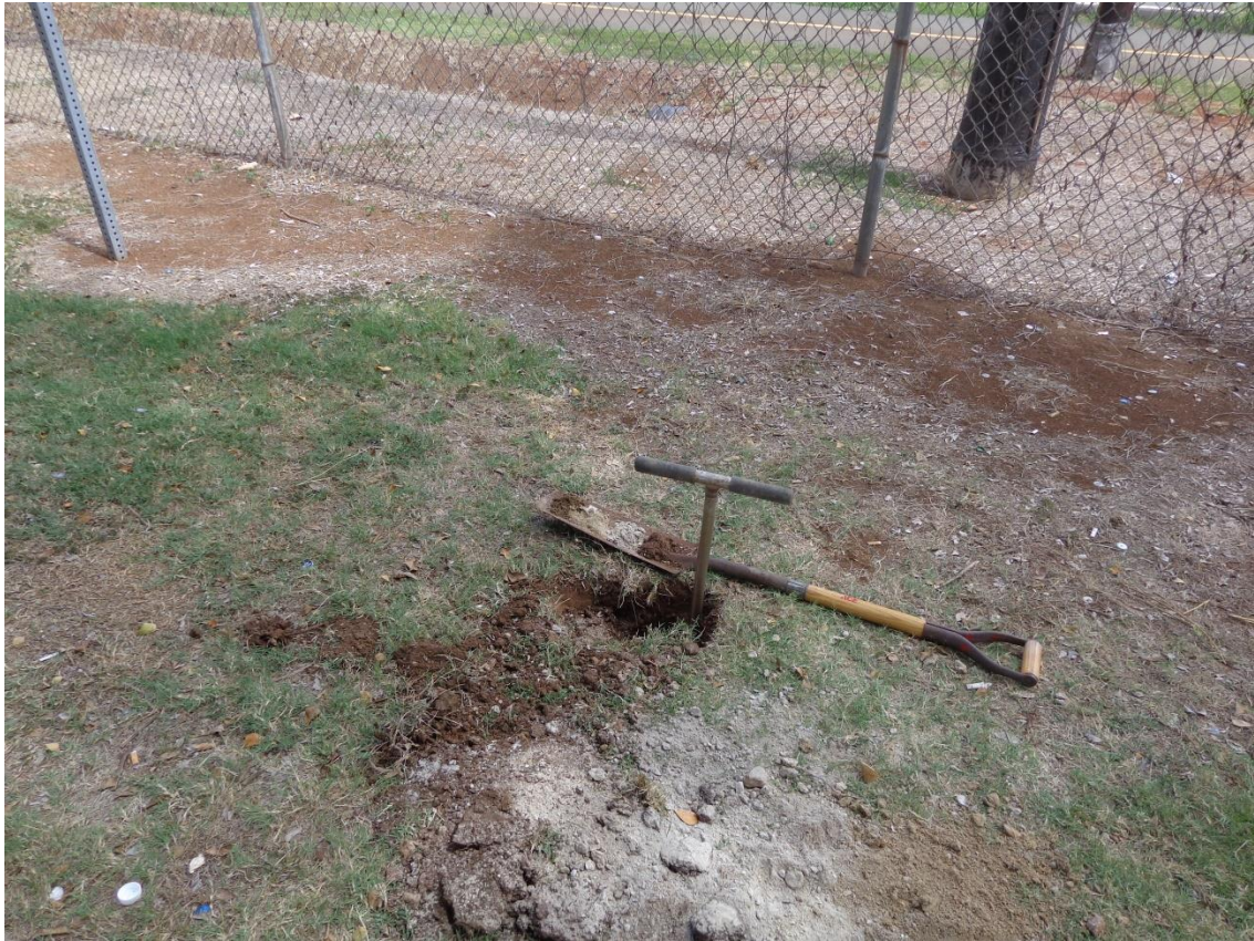
Soil Pit 1A – Southeast corner of the project area, elevation 6.5 feet. Auger shown at 47 inches depth, where struck solid coral layer.
