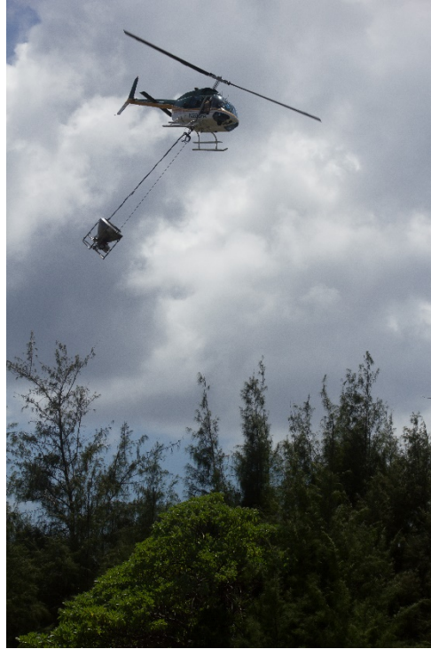
Figure 3. Helicopter rodenticide application using a bait hopper.
