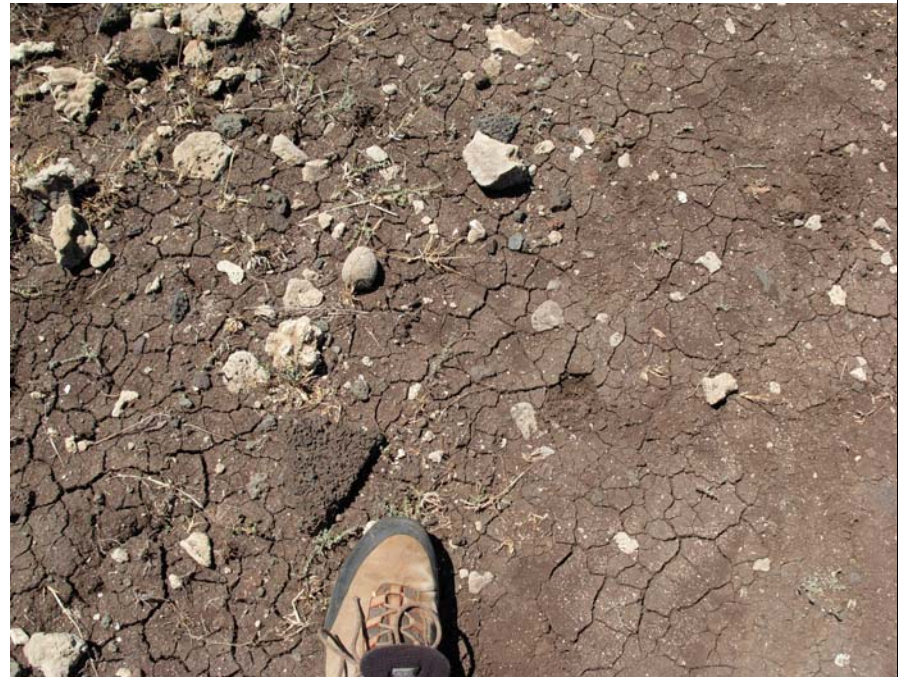
Photograph No. 2: Typical dark brown clay soil with desiccation cracks encountered as generally thin deposits along the western coastline trail northerly of the existing Coast Guard property. Note the embedded coral fragments. (photo 0297)
