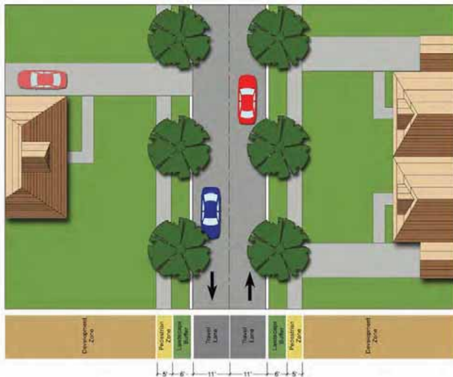
Diagram: Local Road - typical plan and section. Example roads: Residential Development east of Allen Black Road.
