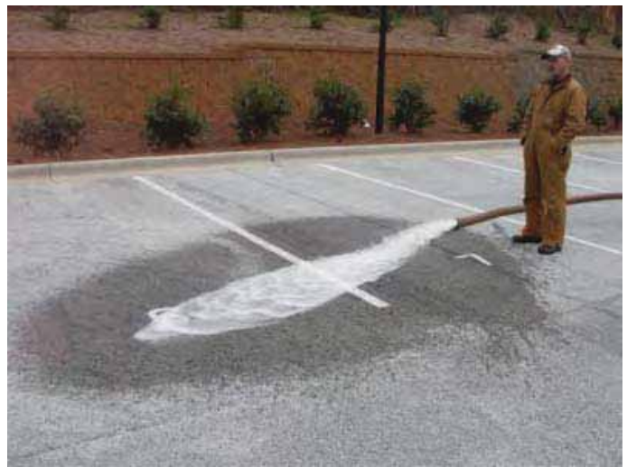
Photo: Pervious concrete can infiltrate large amounts of water. Parking lot in Charlotte, NC, first of its kind in the Piedmont of North Carolina. Designed by Estes Design, Inc., researched and monitored jointly by Estes Design Inc. and UNC Charlotte.
