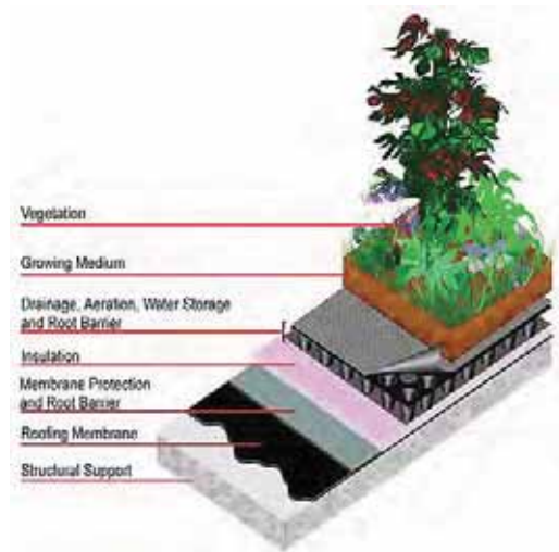
Green roof diagram: green roofs can capture and treat a large amount of stormwater in an area, especially on flat roofs on commercial buildings that take up a lot of real estate. Green roofs are most successful when they are specified early in a building’s construction, to make sure the additional weight from soil and plant material is accounted for in building loads. Square footage in a green roof can be added to open space requirements for LEED certified projects. Low Impact Development Center, Inc.
