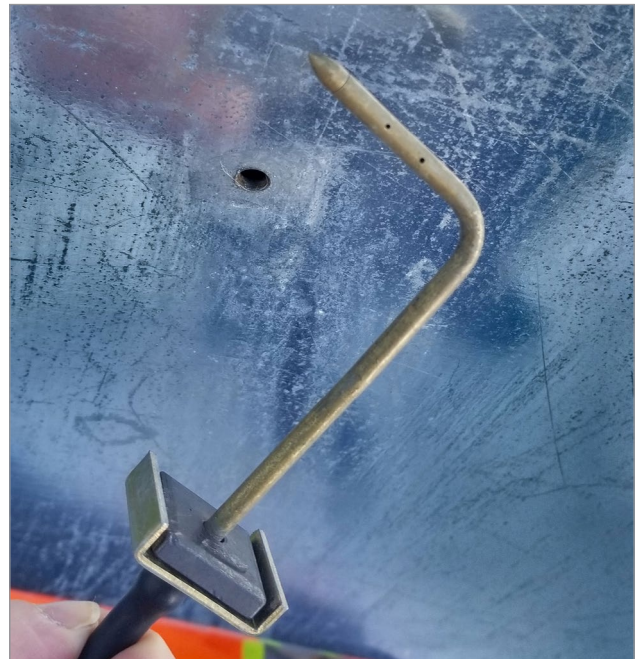
Figure 7. A static pressure measurement tube can be inserted into a small hole in ductwork to measure the air pressure. Source: APS Dineen Farms, Kenilworth ON
