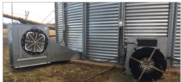
Figure 8. This natural-air drying bin has two fans – a low-speed centrifugal (left) and an inline centrifugal (right) to increase the airflow rate for faster drying.
