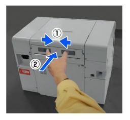
If the duplex feeder is installed, close the rear cover.
