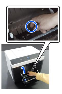
Check that there is no paper or scraps at the back of the inside of the printer.
