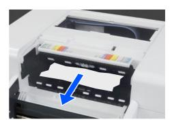
Move the print head unit manually, and remove the paper towards the rear.
