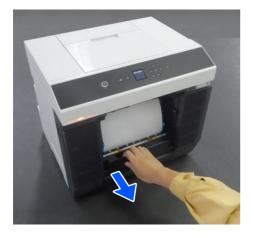
Turn the handle on the left side of the roll paper unit in the direction of the arrow to rewind the paper.
