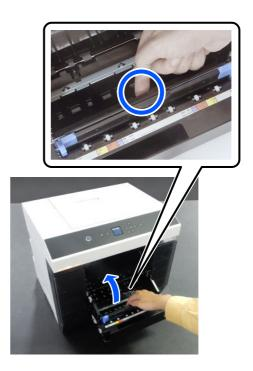
9 Check that there is no paper or scraps of paper inside the printer.
