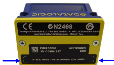
Figure 32 – Apply Replicate Scanner SN Label
