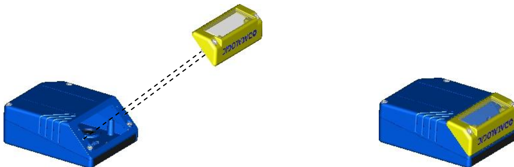
Figure 16 - Mounting a GFC-2020 Deflection Mirror
