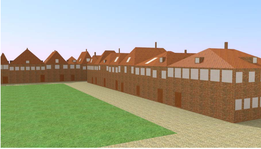
Figure 6.9: Procedural modelling from LOD0 to LOD3. Example of a CityGML model generated with Random3Dcity in conjunction with the existing real-world dataset of 2D footprints of buildings. This setting shows the Beestenmarkt in Delft, the Netherlands. The grammar has been adjusted to match the configuration of the buildings in that setting in order to resemble the reality as close as possible.
