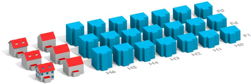
Figure 5.5: An example of a building modelled in 27 representations. The block models are 21 variants of LOD1.2 (3 horizontal references \times 7 vertical references). The three models lined next to the LOD1.2 instances are three variants of LOD2.1 models, differentiated by the horizontal reference. The two models top left are LOD2.3 with references F0 and Fd (LOD2.3 with F1 is not possible). The bottom left is the LOD3.3 model for reference.
