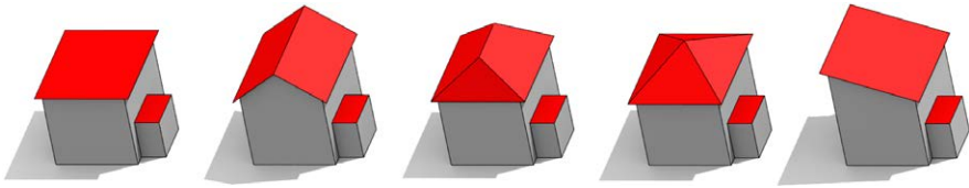
Figure 6.3: Support for different types of roofs. In this example 5 types (flat, gabled, hipped, pyramidal, and shed) are fitted on the same building body, with the automatically adjusted walls. This image illustrates the LOD2.3, and it also features an example of a building part.
