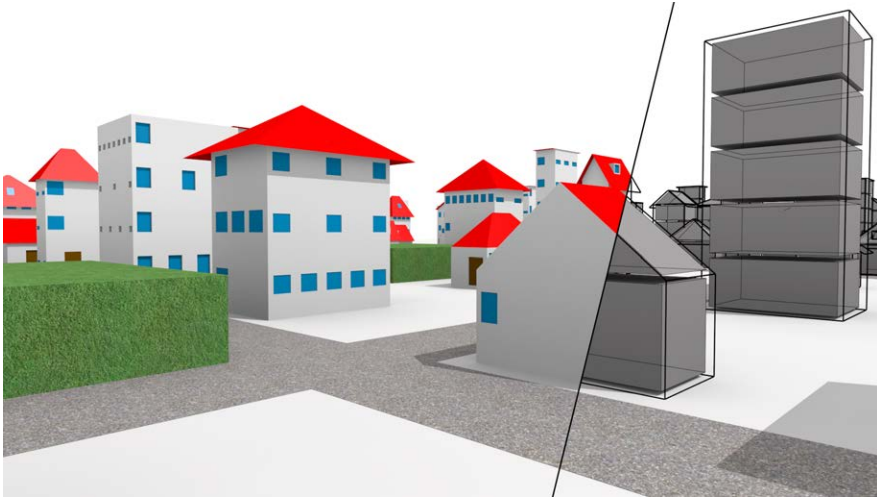
Figure 6.8: A composite street view of a dataset generated by the engine. The image shows the vegetation (park), street network, and the basic indoor representation of buildings (a solid representing each storey).
