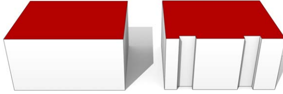
Figure 3.7: Two buildings modelled in different feature complexity. The wall surface (white) and top surface (red) at the finer LOD (right) are modelled more precisely due to the finer feature complexity requirement.
