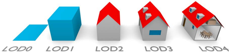
Figure 1.3: The five LODs of the OGC CityGML 2.0. The standard attempts to assign standardised classes to generally differentiate grades of 3D data. The geometric detail and the semantic complexity increase with each level. This LOD categorisation is well known in the 3D GIS community, however, it is not without shortcomings, and it is therefore thoroughly discussed in this thesis.
