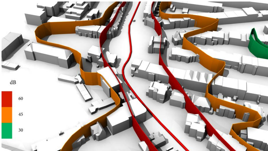
(b) Estimating noise pollution. This is an illustration of noise from a planned tram track (red line) in an urban environment. Owing to analyses such as this one it is possible to predict how many citizens will be affected by noise if the tram line is built. This is a 3D analysis because noise propagates in 3D, and the analysis enables us to determine not only how many buildings are affected by excess noise pollution, but also which floors will be affected most.
