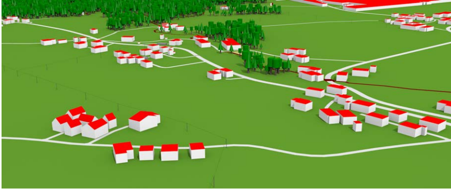
Figure 12.1: 3D building models of heterogeneous lineage within the same dataset. Example of a 3D model of a village in Austria obtained with crowdsourcing. In reality, almost all buildings in the area have pitched roofs, however, they are modelled only in a few buildings on the left (LOD2). The rest of the buildings are represented by simple block models (LOD1). 43
