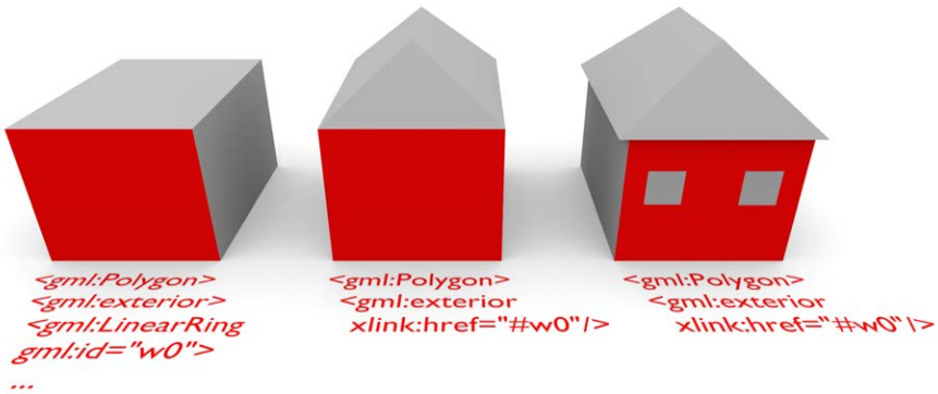
Figure 8.2: The rationale of the method to link multiple LODs. If two or more geometries are found to correspond, links are created. In this case two polygons (walls) are identical in two LODs. However, in one LOD the polygon has a hole, hence only their exterior rings are linked. How and where to establish the links while balancing the maximisation of links and the topological structure is the main concern of the consolidation process.
