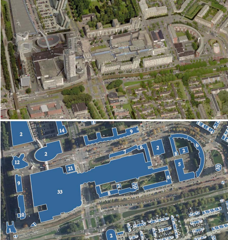
Figure 7.13: Example of a footprint covering multiple buildings of significantly different heights. The labels represent the number of storeys for each footprint, which we have used to predict heights, and in this case resulted in erroneous predictions. In cases such as this one it is ambiguous to discuss building heights. 25
