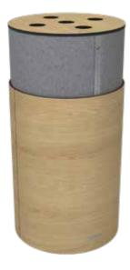
**Vari Bass Ultra** is designed for use in any Hi-Fi room. Made from wood and high-density acoustic foam, the bass trap can be tuned between 50Hz-100Hz by simply rotating its wooden top (which has a series of resonant pots) until the problem disappears. A scale is included to show the exact frequencies on which the Vari Bass Ultra is acting. The unit's stand-alone structure enables it to be repositioned as required and used in different rooms.
