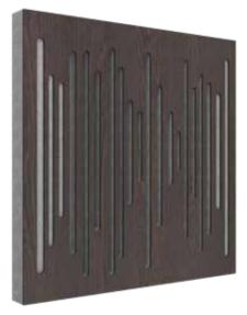
Simulating a QRD and MLS sequence the **Wavewood Diffusor Ultra** is an ideal solution to those who search balanced sound ambiences that simultaneously control the exceeding energy in a room, flutter echoes, and still maintain a living and bright sound. It is particularly effective in treating medium and high frequencies.
