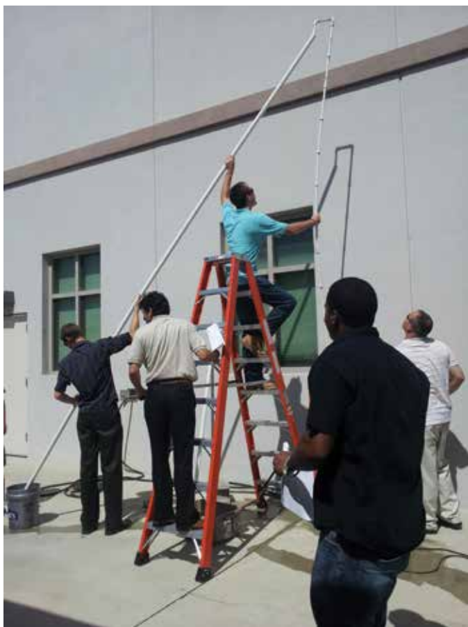
Photo 1. Florida Gulf Coast University students enrolled in CWR 3201, Engineering Fluid Mechanics, use the outside of their hybrid laboratory and lecture building to aid their measurement of the ability of a water pump to lift water through a narrow PVC pipe.
