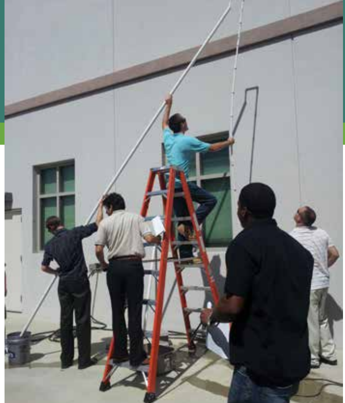
160 Students use the outside of their hybrid laboratory and lecture building to aid their measurement of the ability of a water pump to lift water through a narrow PVC pipe.
