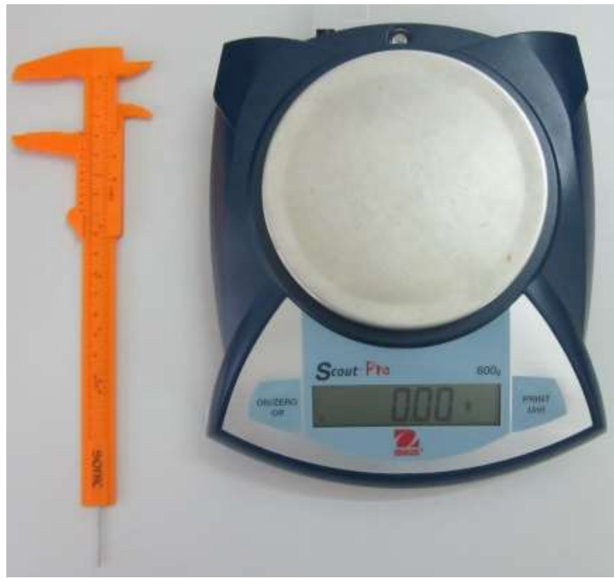
Figure 4. Panme ruler on the left and electric weight scale on the right used in biological samplings
