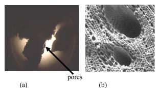
Figure 6: Microscopic view of activated carbon, under light microscope (a) and under electron microscope (b)
