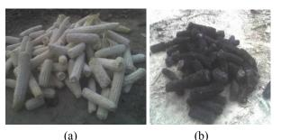
**Figure 3**: Maize cob residue being carbonized (a), carbonized maize cob residue (b)
