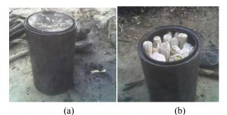
**Figure 2**. Perforated lid of an empty tin (a), raw maize cob residue packed for carbonization (b)
