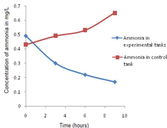
**Figure 10.** Ammonia concentration profile in the treatment and control during a period of 9 hours.
