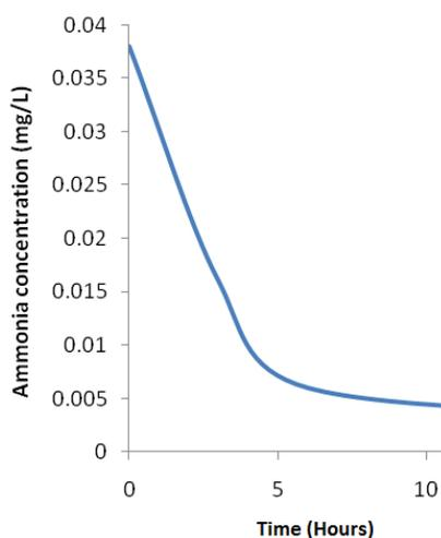
**Figure 8.** Ammonia concentration profile in a period of 9 hours following the application of 20g of activated carbon to the treatment tanks.
