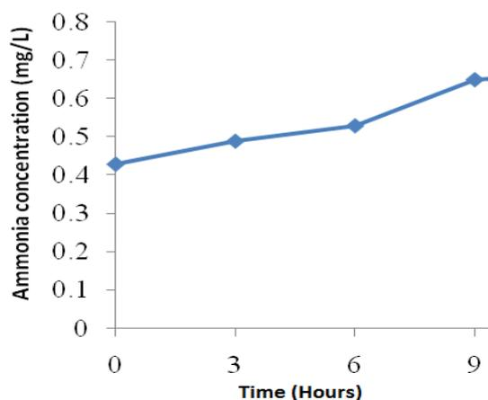
**Figure 9:** Amount of ammonia in the control tank during a period of 9 hours.
