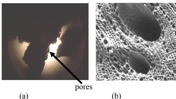
**Figure 6:** Microscopic view of activated carbon, under light microscope (a) and under electron microscope (b)
