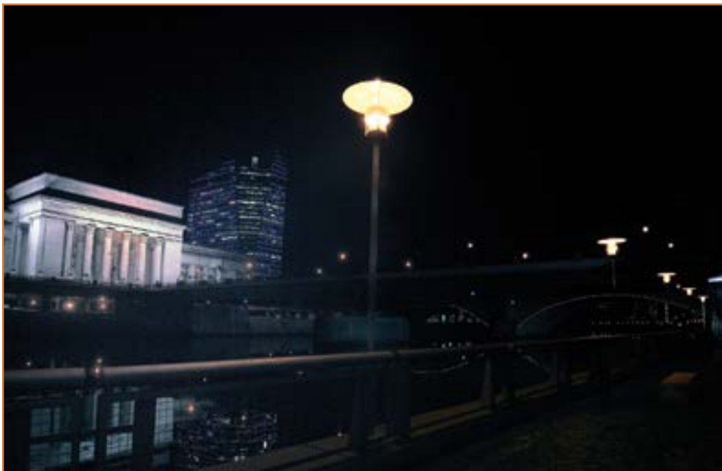
Figure 9.6 Lamp design attractive to bridge spiders. Overhanging reflectors shield webs from rain and anchor them. These lamps line the east bank of the Schuylkill River.
