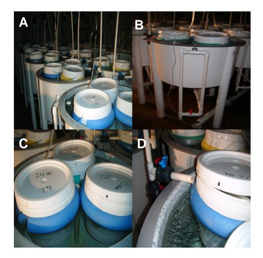
**Figure 3.3.** Spawning experiment 2 aquaria set up with A) Three 10 L buckets positioned within each tank B) Individual aquaria tank showing water outflow and air filtration lines C) Positioning of three buckets within each tank with bucket number and treatment times displayed on lid and D) Water inflow into each aquaria.
