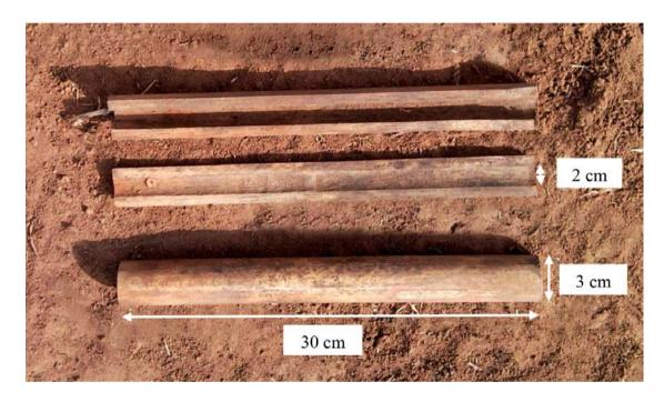
Figure 2-6. Wooden dowling artificial burrows. The upper two images are the two halves of a burrow that has been cut open to reveal the internal structure.
